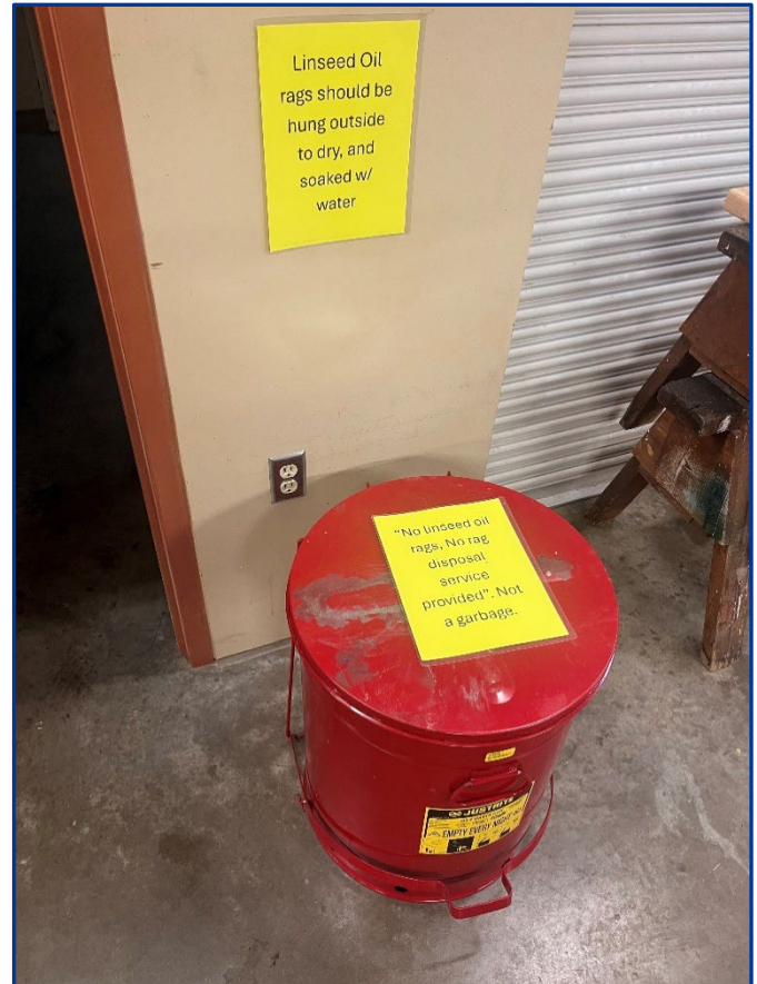
The Justrite rag can back in place in the Kawishiwi Ranger Station’s wood and paint shop—with the new “no linseed oil rags” signs posted.
